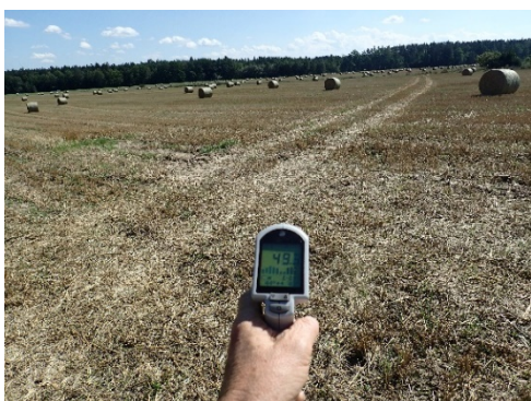
Picture 2: Large-scale cultivation of biofuel crops in the Czech Republic. Measured values of solar radiation, surface temperature and air humidity on a harvested field show that incoming solar energy ( 823\text{W/m}^2 ) is transformed mostly into sensible heat ( 49.5\text{ }^\circ\text{C} ) and dries out the landscape.
